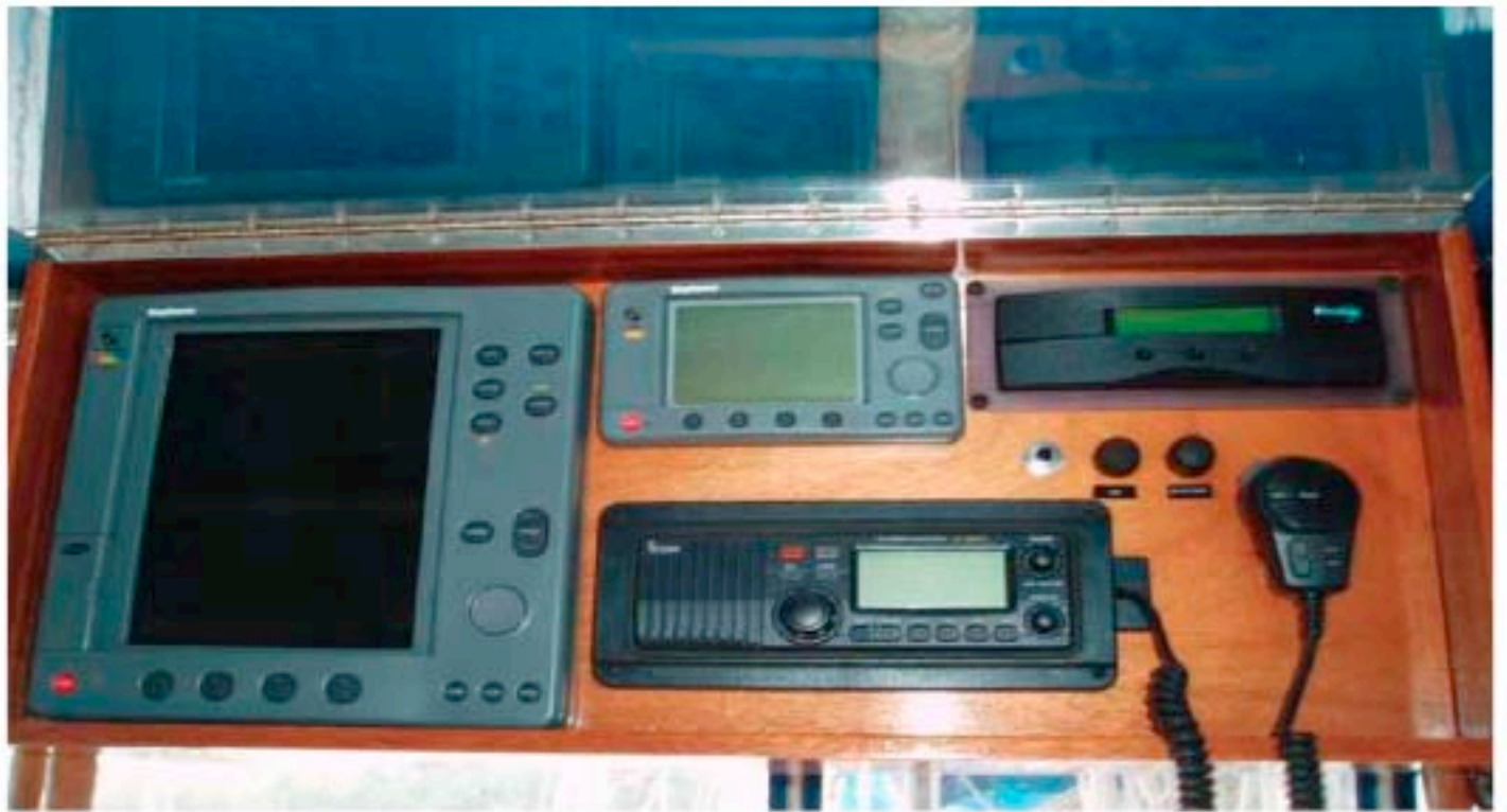
Instruments above helm. Lockable lexan cover. L to R. Raytheon RL80C radar/plotter. Raytheon RN300 GPS, GyroTrac compass. Horn buttons ICOM M-127 VHF
